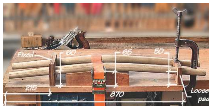
▲ Pic. 2 Hold the bending jig in the vice with a longitudinal batten screwed to its underside
